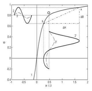
Fig. 1. Theory of saturation controllable reactor
