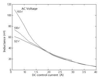
Fig. 9. Control characteristic of the reactor
