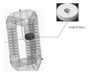
Fig. 5. Structure of three-phase controllable reactor
