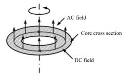
Fig. 4. Fluxes in the orthogonal core
